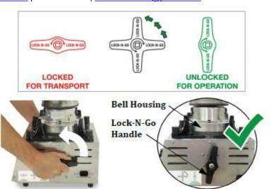
Step 2: Lock-N-Go® handles are used for transport. Rotate both handles to a vertical, UNLOCKED, position for use. This allows the bell housing to "float" freely on the springs during operation. DO NOT operate with handles in the transport position.
