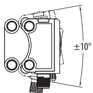
3. After adjusting the sensor to the desired position, secure the mounting bracket with the two M3 screws and washers.
